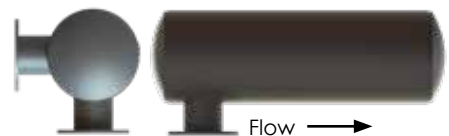
Side in 6 o'clock, Side Out 9 o'clock
